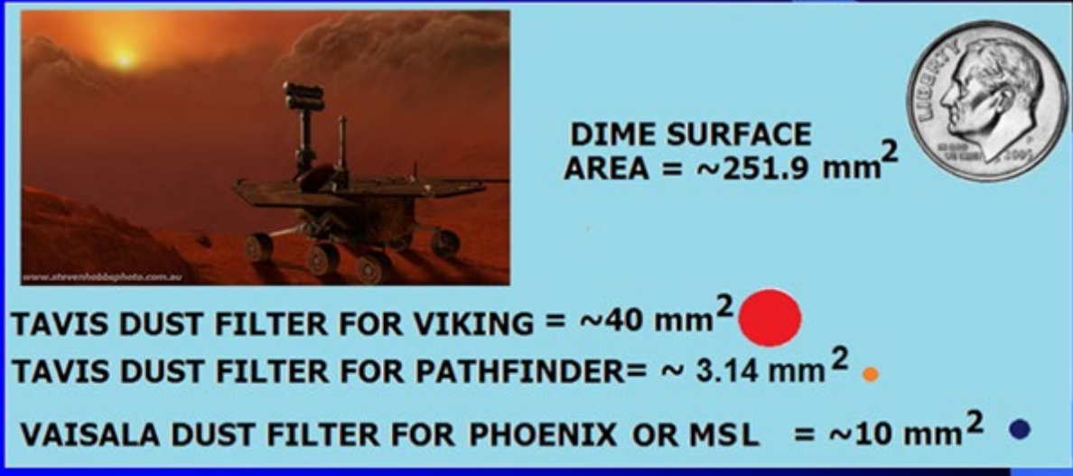
Figure 7-12 above: Relative size of dust filter for landers on Mars. 2 mm diameter of Mars Pathfinder (MPF) tubing from Seiff et al. (1997). On Figure 7-13 below, the top transducer is for Phoenix. Note the tiny dust filter shown under Praw (adapted from Doc. No: FMI_S-PHX-BAR-TN-00 FM-00 Revision 1.0 dated 2009-02-26). The report is entitled The Time Response of the PHOENIX Pressure Sensor . An area of concern for clogging by dust is highlighted. The photo on the right is adapted from http://www.space.fmi.fi/phoenix/?sivu=instrument . The bottom pictures are for MSL.
